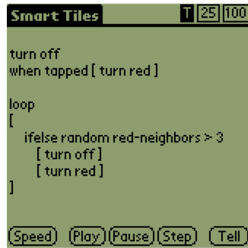
Figure 9: A screen view of a handheld device being used to reprogram, textually, a set of SmartTiles.
